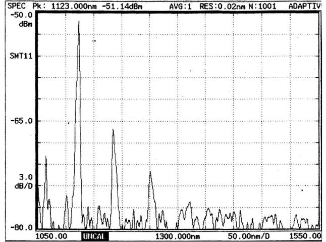
Fig.6 The spectrum of multi-order Stokes wave without  $M_1$
