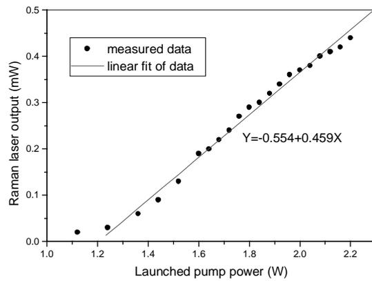
Fig.10 The graph of laser output verse launched pump power
