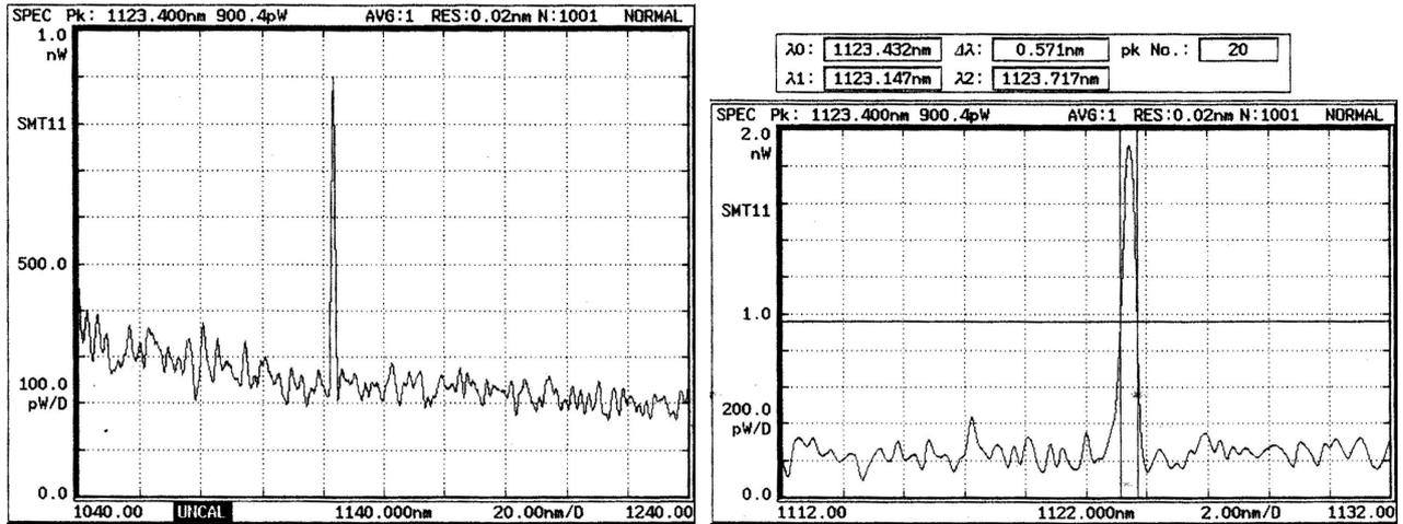
Fig.7 The spectra of the first-order Raman laser with two mirrors (FWHM is measured in the right)
