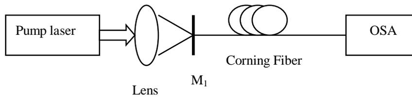
Fig. 1 Schematic configuration of the experimental setup
