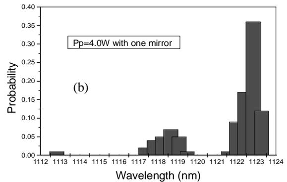
Fig.5 The probability of different modes at different pump power of (a)3.0W (b) 4.0W
