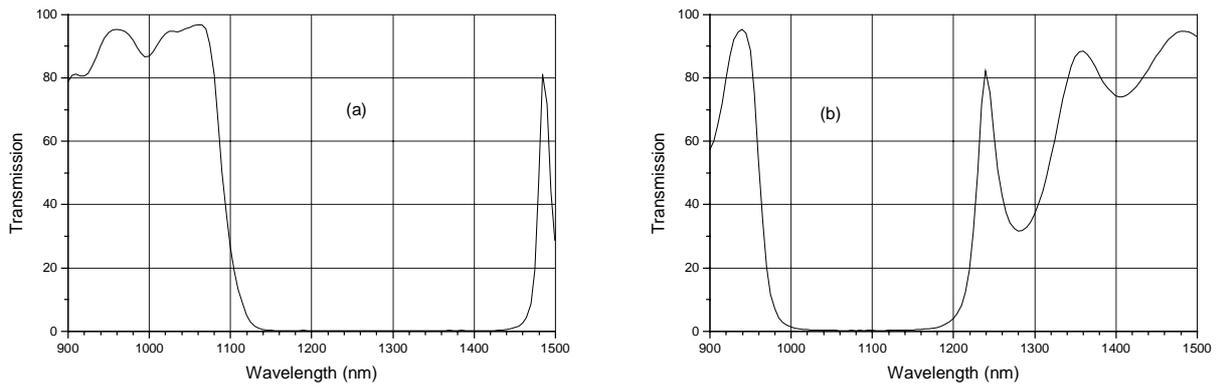
Fig.2 Transmission spectra of mirror (a)  $M_1$  and (b)  $M_2$
