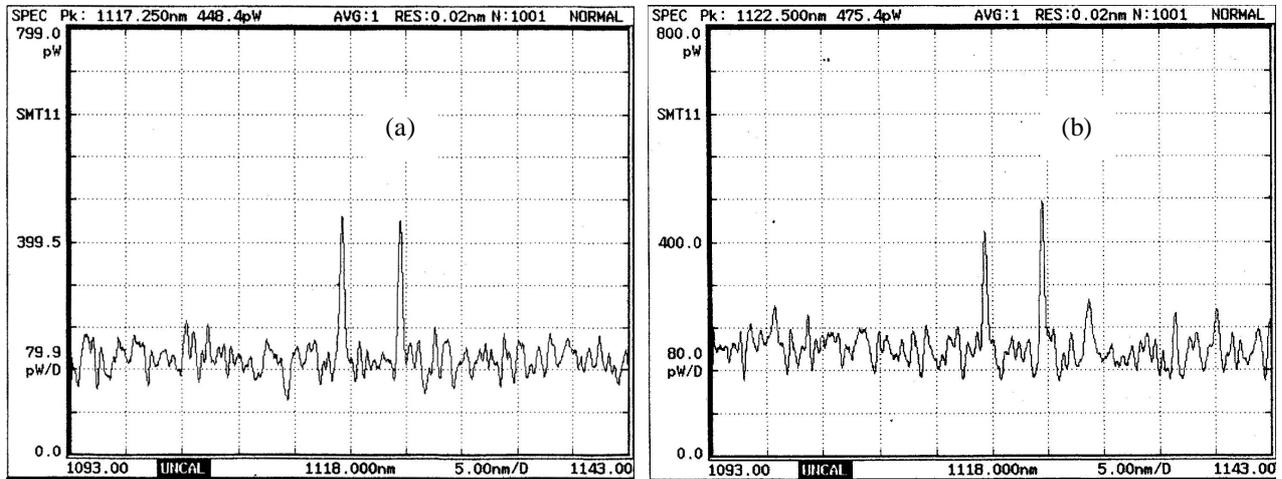
Fig.8 Mode competition for the first-order Raman laser with two mirrors centered at (a) 1117 nm (b) 1123nm
