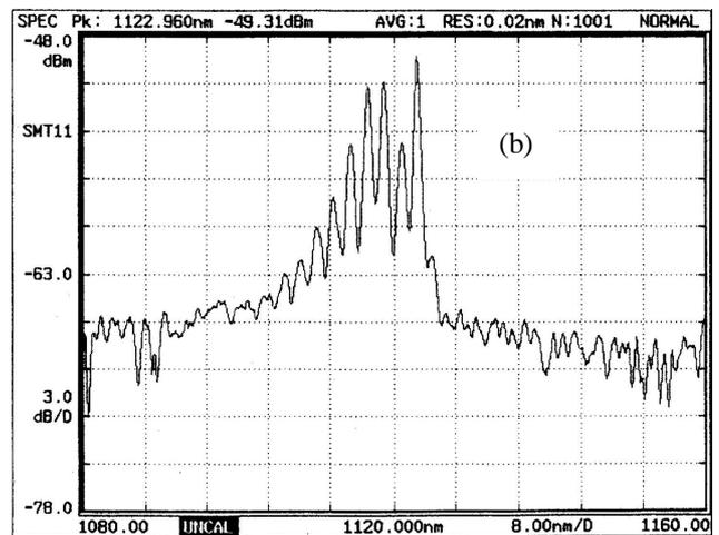
Fig.4 Mode competition for the first-order Raman laser centered at (a)1117 nm (b) 1123nm
